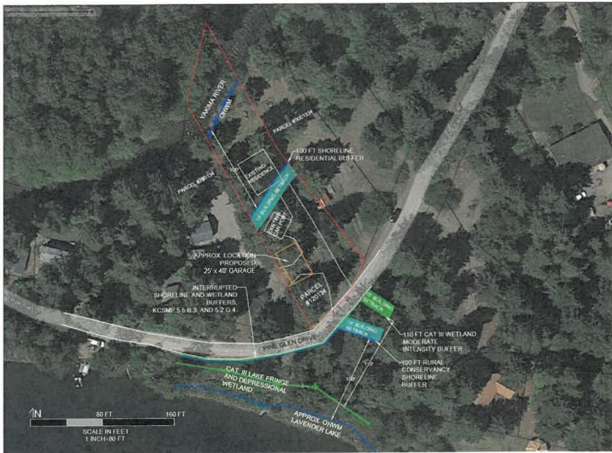
Figure 2. Location of the proposed garage in relation to critical areas and their associated buffers.
